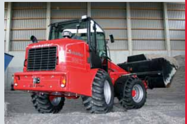
Full floating axle in rear for more stability and higher excavating force.
