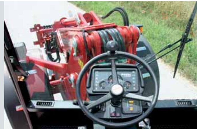
Clear view due to low swing coupling.
