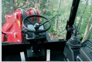
Hydraulicly pre-controlled valves make work with a 9100 Z a pure pleasure. The absolutely delicate dosage of the work hydraulics by means of one hand joy-stick and exactly defined pressure points aren't only more comfortable but also safer. The spacious and comfortable cabin keeps the driver fit longer.
